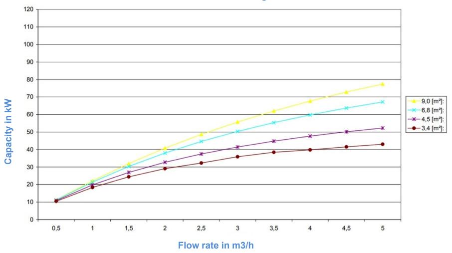
Each tank with this heat exchange system has a capacity of approx. 120 kWatt at a delta T of 10k. This means a total of approx. 240 kWatt at a flow rate of 3,5 m3/h.
